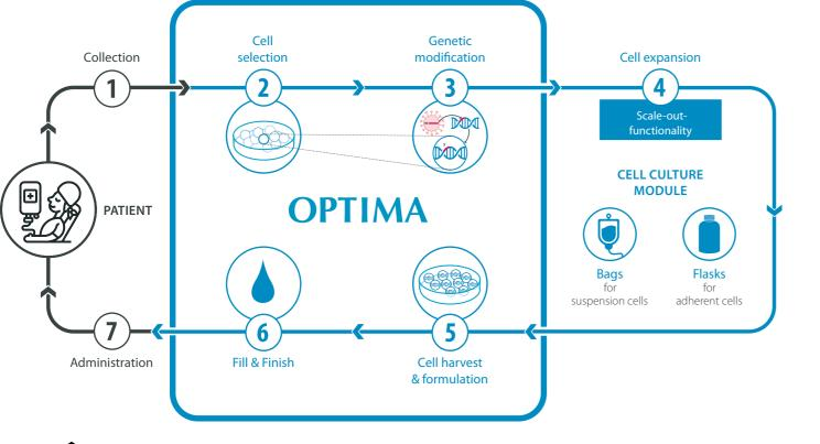
In the Stuttgart/Heidelberg ProCell for Patient model, essential steps (blue) in the production of cell therapeutics are performed in an isolator in a fully automated process. The prototype will be installed at the Robert-Bosch-Krankenhaus in Stuttgart.
