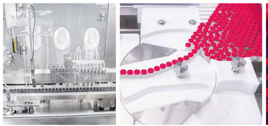
High speed, precision filling: Up to 24,000 vials per hour are processed by the system. 100 percent of the containers are inspected by an in-process control.
