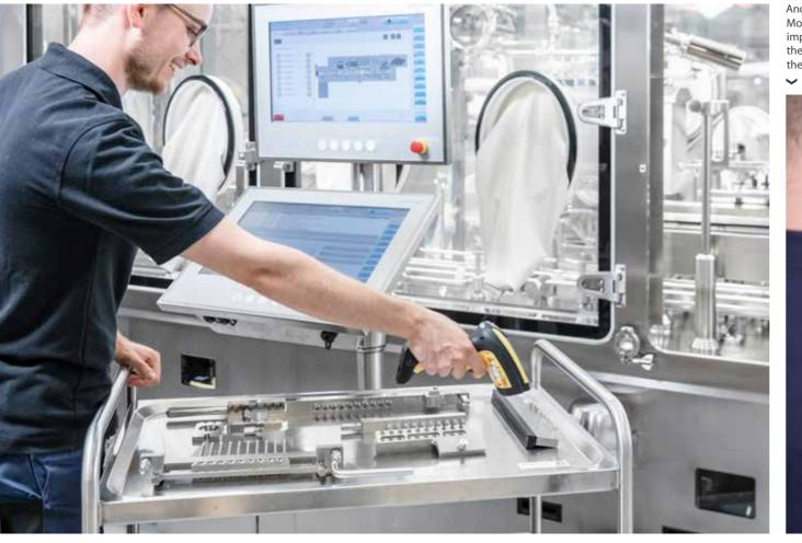
Another added benefit of Video Monitoring: Operators have an improved overview of the system as the cameras transmit live images to the HMI.
