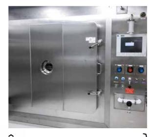
The freeze dryer chamber with door can be seen. Bachem is now using freeze drvers from Optima for the first time.
