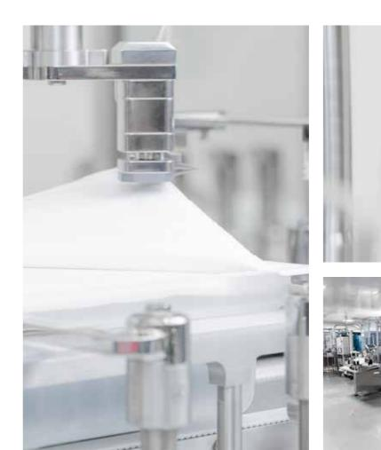
The removal of the sealed foil of the tub and the removal of the Tyvek cover is done fully automatically.
