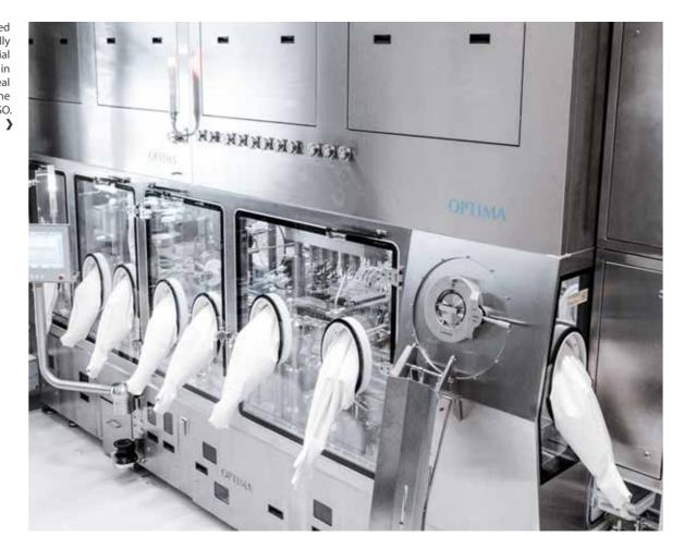
show part of the overall complex isolator technology. The HVAC unit (HVAC: Heating, Ventilation and Air Conditioning) is located, almost invisibly, above the isolator on the technical floor. If it were possible to dispense with the large HVAC unit and extensive piping, it would be feasible to significantly reduce the amount of work involved in isolator tallation and commissioning
