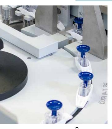
At USV India, a second Optima system assembles safety devices. The syringes are also labelled.
