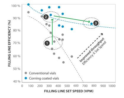
Figure 3: Filling line efficiency tends to rapidly decline with increasing line operating speed when using conventional vials. Corning Valor<sup>®</sup> vials maintain high line efficiency relative to conventional vials, even as line set speed is significantly increased. (Cornina)
