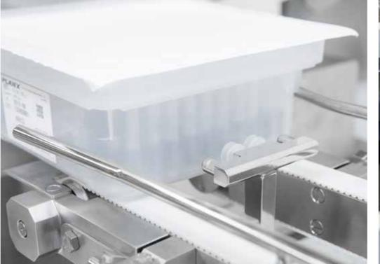
Flexible filling processes for readyto-use syringes syringes and vials. Depending on the batch sizes, the number of filling points can also be modified.
