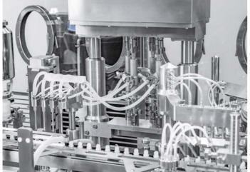
Four headed filling sytems: Concealed on the left are the stacked peristaltic pumps. Also installed rotary piston pumps to process viscous products.
