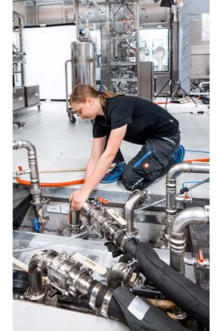
The media troughs running in the floor of the CSPE centers can be quickly connected to all line sections. This means that commissioning can take place under realistic production conditions.
