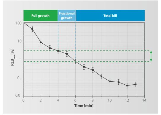
Safe aseptic processes in isolators require a solid cycle development. Parameters for the decontamination process during cycle development are first defined, then gualified and validated on a regular basis. To date, only biological indicators are used. Recently Enzyme indicators were introduced that also react to H<sub>2</sub>O<sub>2</sub> in a timely manner and are conditional to dosing volume and might have additional benefits.
