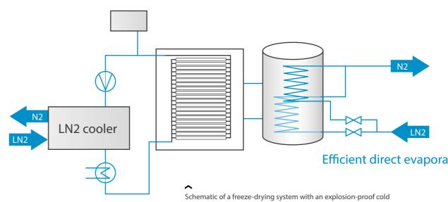
cascade system. Both components - freeze-drying chamber with shelves and ice condenser - receive cold air from a central cooling system via heat exchangers and fluids in their own circuits.
