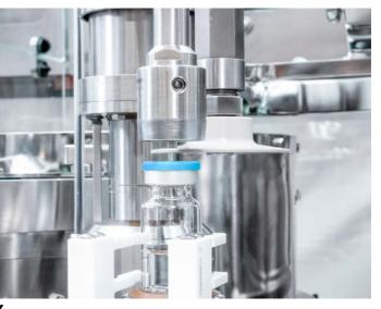
Highly precise dosing system, exact filling volume: If a fill volume is inaccurate, the container is immediately refilled instead of rejected - the so-called "re-dosing on request".
