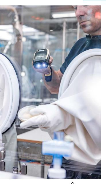
Using a new digital solution from Optima Pharma, agar plates can be scanned and unequivocally assigned. In addition, timing functions are also integrated.
