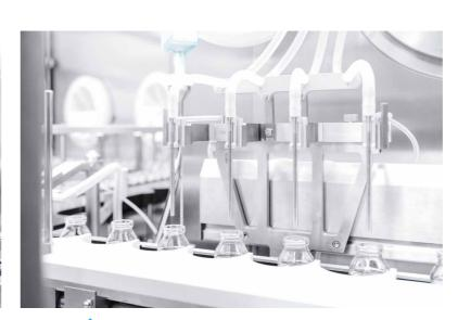
Up to 5,000 vials are processed per hour. Product saving functions make optimal use of the available quantity of drugs.
