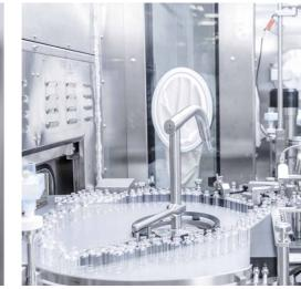
After the sterilization tunnel, there is a transition to the isolator-protected filling area.
