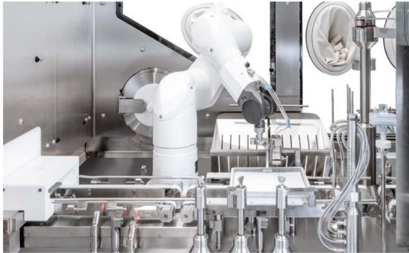
← The pre-sterilized and nested RTU containers are prepared for further processing. A robot peels off the Tyvek and then removes the lid liner.
