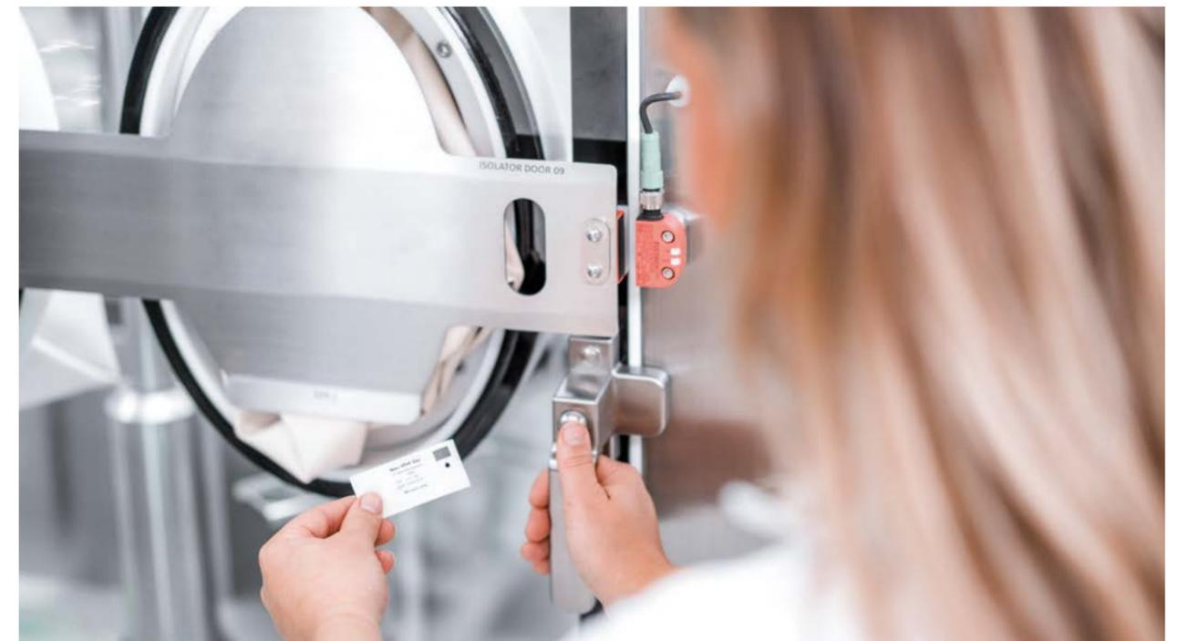
↑ As part of the preliminary cycle development at Optima Pharma, indicators were used to identify best-case and worst-case locations in the isolator-protected area.
