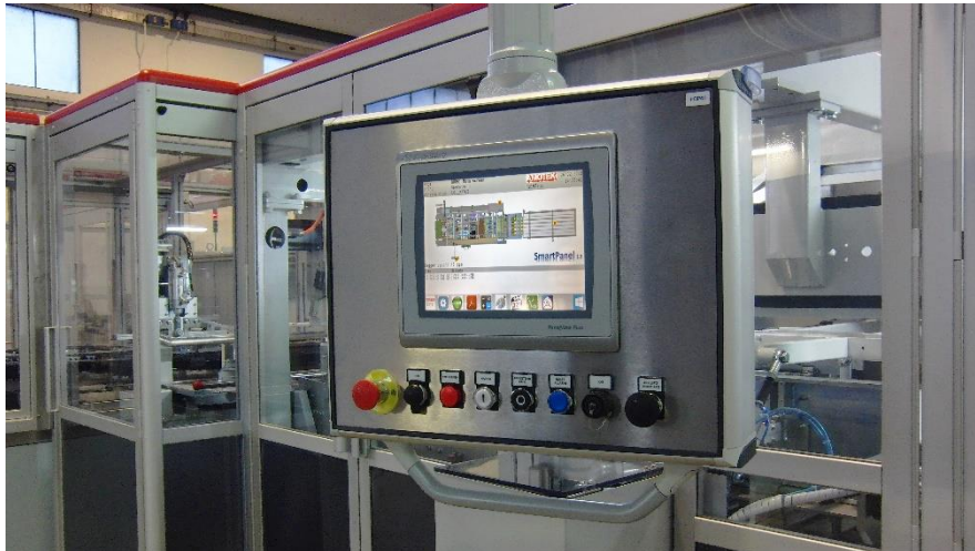
The AMOTEK PB192 records all process data and machine functions and displays them on a big new high-resolution monitor.
